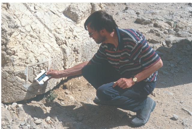
Fig. 12: Profile measurements – limestone statues.
