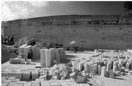
Fig. 2. (a) Modern buildings in Globigerina Limestone show that to this day this limestone is still one of the most important building materials in Malta. (b) This quarry, which is still active today, shows the extraction of Globigerina Limestone. The limestone blocks, here exposed to rain and sun for a short period, were previously left for much longer and led to a hardening of the stone surface.
