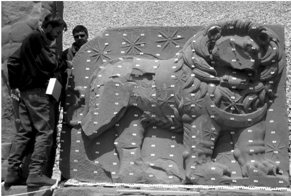
Figure 7: Ultrasonic measurements. Lion horoscope, Nemrut Dag / Turkey.
